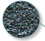
Microporous structure Pore size ~160 μm
